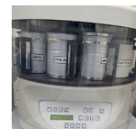
Automatic tissue processor (Leica TP1020)
